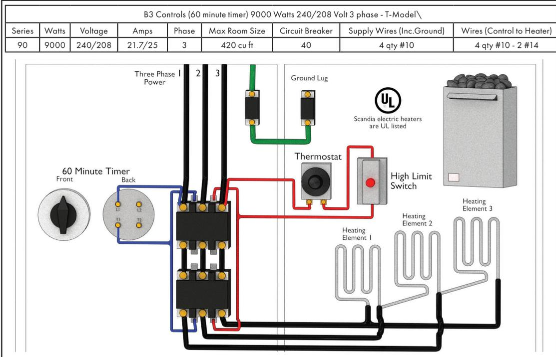
For supply connections and control panel to heater connections, use wires suitable for at least 194° F (90° C)
