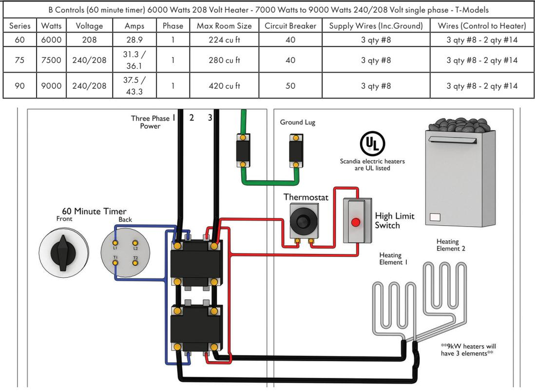
For supply connections and control panel to heater connections, use wires suitable for at least 194° F (90° C)
